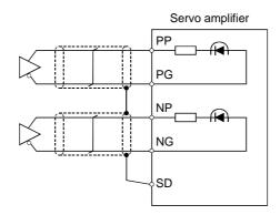
The explanation assumes that the input waveform has been set to the negative logic and forward and reverse rotation pulse trains (parameter No.21 has been set to 0010).
